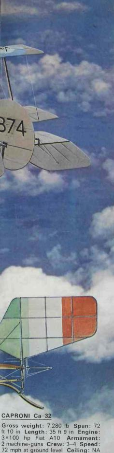
72 mph at ground level Ceiling: NA Range: 340 miles Bomb load: 200 lb
