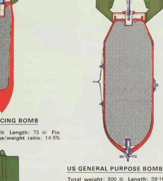
Total weight: 500 lb Length: 59.16 in Fin width: 18.94 in Charge/weight ratio: 51%
