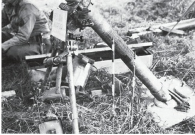
An 80mm German mortar, the Granatwerfer 34 , which had a maximum range of 2,400m.
