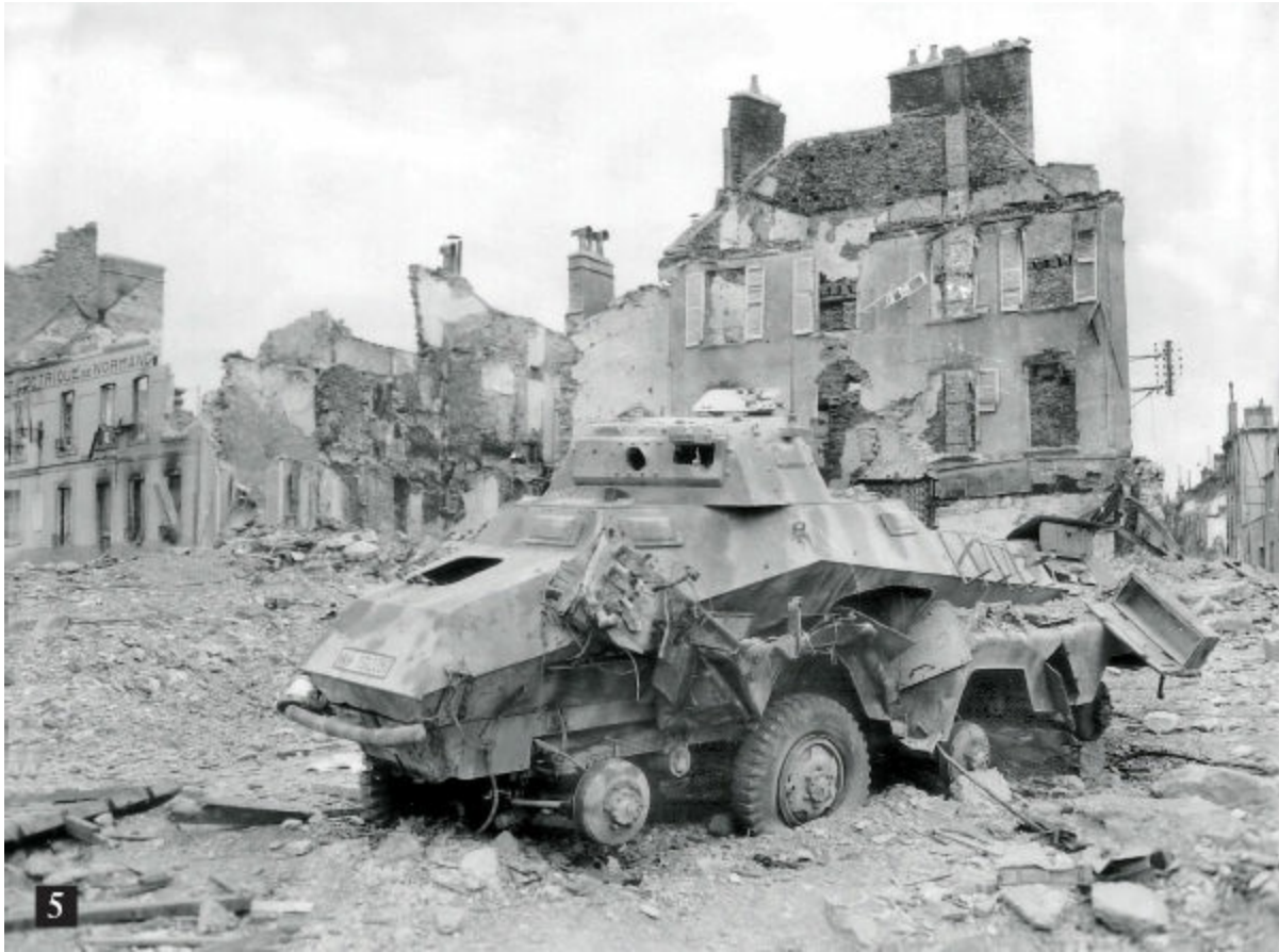
5. A little further ahead, this armoured German reconnaissance vehicle has been put out of action due to the intense shelling. It is a Schwerer Panzerspähwagen (8 Rad) (Sd.Kfz 231); an 8-wheeled reconnaissance tank with four crew and a 2cm KwK 30 and MG34 gun. It could consume 45-50ltrs of fuel per 100km.
