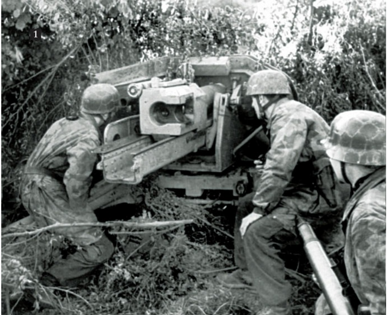
1. Often hidden in the corner of a hedgerow, the 7.5cm Pak 40 anti-tank gun was particularly effective against American tanks. Here, the men can be seen adjusting the sight while the soldier on the right (not wearing a paratrooper's helmet), stands ready with a 75mm shell, capable of piercing 32mm armour from a distance of 500m. (BA 1011/582/2120/7.)
