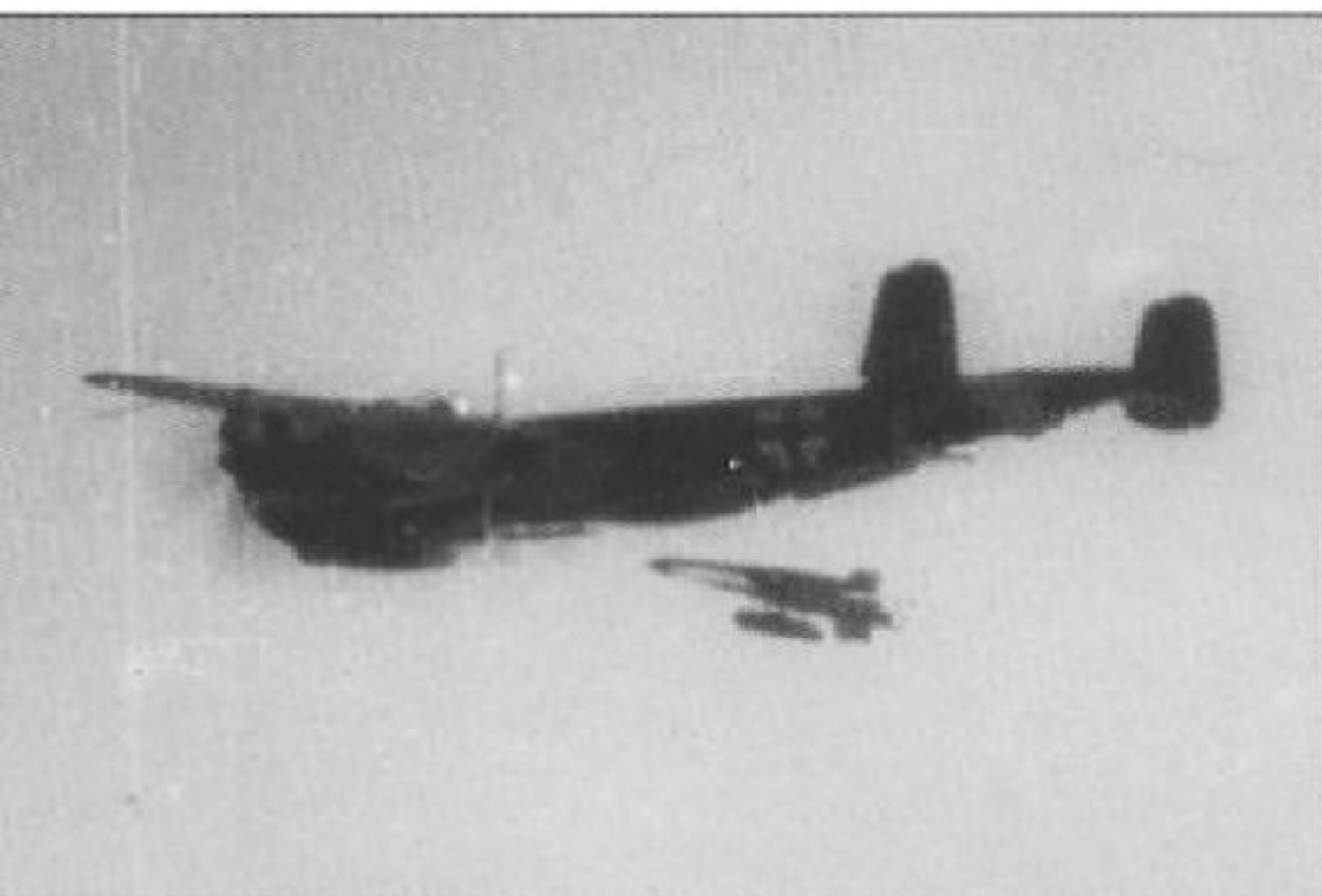
Above: The Dornier Do 217 was the aircraft of choice for the deployment of the Henschel Hs 294 anti-ship missile. Perhaps 1450 of these sophisticated guided missiles were ordered but few were completed.
