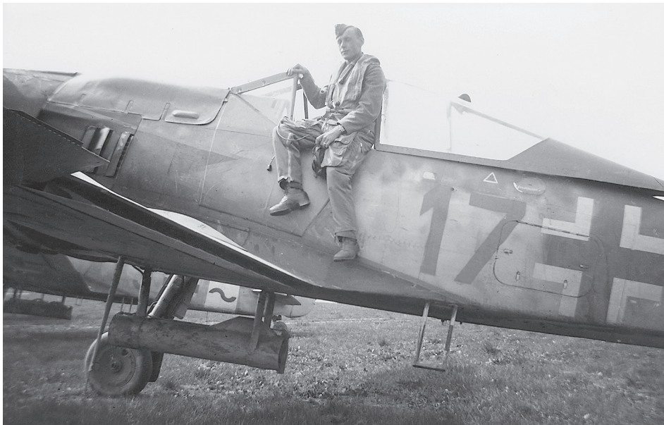
Unteroffizier Willi Unger of 12./JG 3 photographed with his Fw 190A-8/R2 'Yellow 17' at Barth during trials with the Krebsgerät , a fuselage-mounted, rearward-firing 21 cm mortar. The intention was that a pilot would make a frontal attack against a bomber Pulk , and as he passed overhead, would fire the mortar. The weight of the device adversely affected speed and manoeuvrability, and posed a risk to other Luftwaffe fighters following behind. The weapon was abandoned. (Unger/Forsyth)
