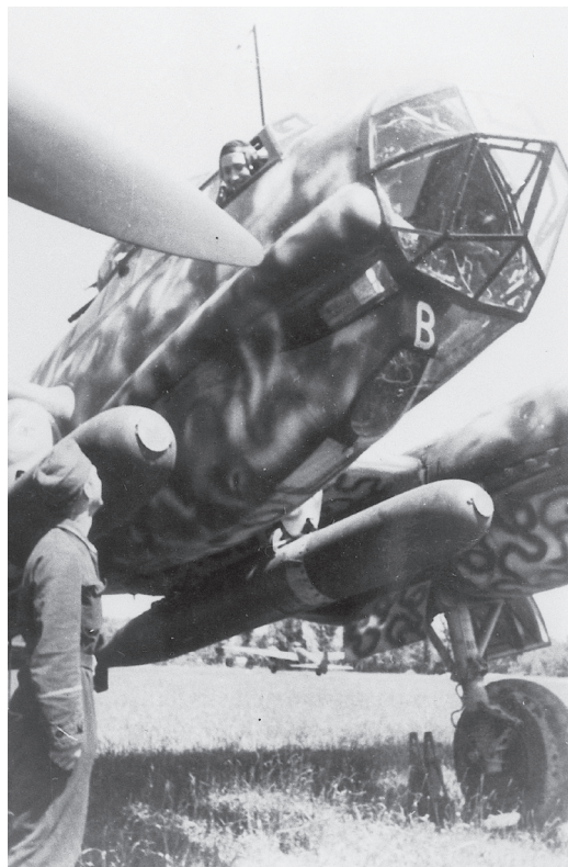
Ju 88A-17 'White' or 'Yellow B' of I./KG 77 loaded with two LT F5b torpedoes in what is probably a posed photograph in southern France in the summer of 1944. Note the 'meander' over-water camouflage pattern which extends over the entire fuselage and engine nacelles. (Goss)
