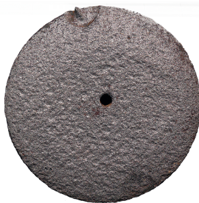
ABOVE The lower, covered end of the barrel has a 4 mm drilled hole for the electric ignition wire. (Hans-Hermann Cammann/JG 400 archive)
