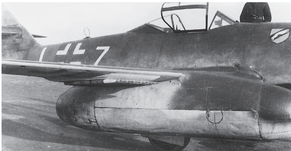
Twelve R4M rockets have been loaded onto the launch rack carried by this Me 262A-1a of 9./JG 7. Visible is the running fox emblem of the Geschwader . [Forsyth]
