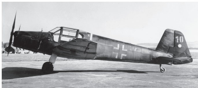
Bücker Bü 181C-2 Wk-Nr 502167 of the 3. Panzerjagdstaffel based at Kaufbeuren in April 1945. The aircraft was photographed at Zurich-Dubendorf, having had its Panzerfaust wing racks removed shortly after being flown to Switzerland on 18 April 1945 by its defecting crew of Unteroffiziere Hans Ficker and Werner Diermayer. Note the firing sights fitted to the top of the cowlings. (EN Archive)
