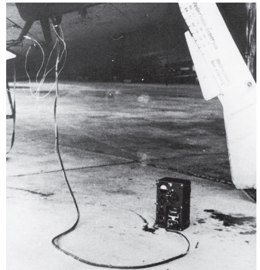
Testing the firing release mechanism on the ETC 70 rack beneath the starboard wing of an Fw 190. (Forsyth)
