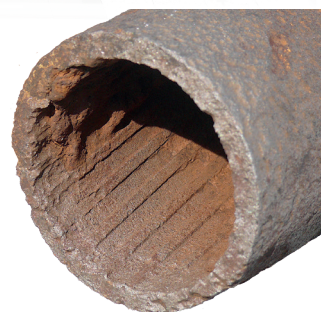
ABOVE Internally, the barrel of the SG 500 had 24 spiral grooves. (Hans-Hermann Cammann/JG 400 archive)
