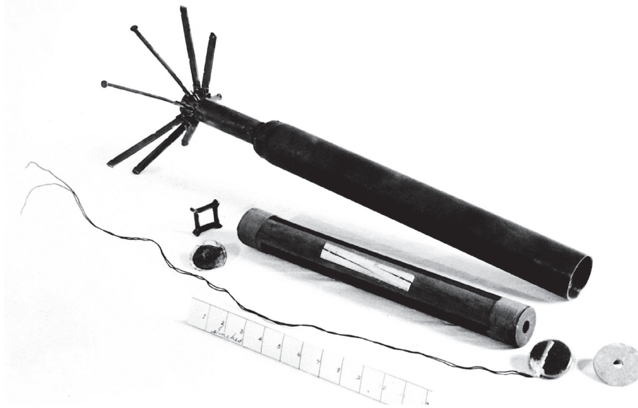
The component parts of the R4M rocket less the fuse and warhead, but showing the extended stabilising fins, ignition wire and the removed inner propellant chamber. (Forsyth)
