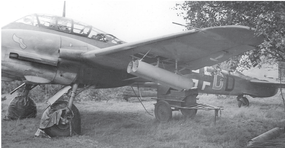
Me 210A-1 Wk-Nr 2102251 2N-DD of ZG 26 has been fitted with four 21 cm air-to-air mortar tubes intended for breaking up and dispersing USAAF bomber Pulks . The tail fin and rudder have been painted white, probably for tactical and recognition purposes during operations in the air. (EN Archive)
