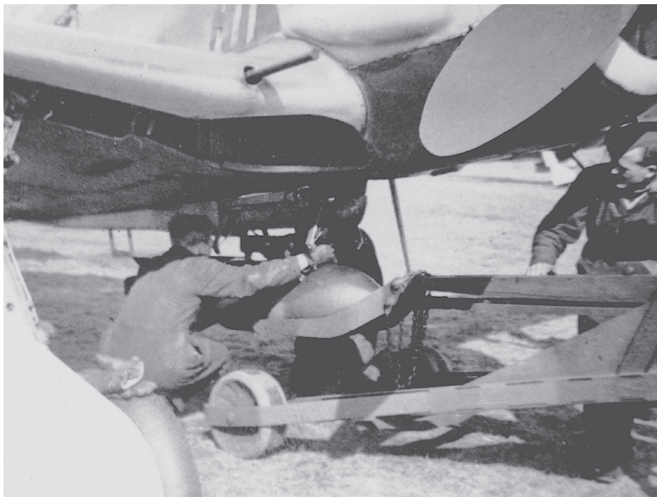
Armourers load an SC 250 bomb from a hydraulic trolley to the underside of an Fw 190A-4 of I./JG 1 based in the Netherlands in the spring of 1943. [EN Archive]
