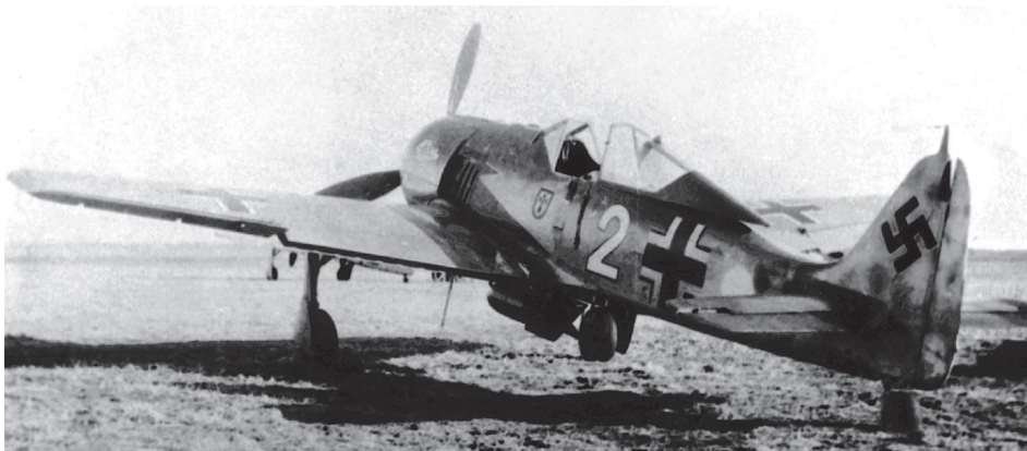
Fw 190A-4 'White 2' of I./JG 1, probably photographed at Deelen in the Netherlands in 1943, has been fitted with a 250 kg SC 250 bomb for air-to-air bombing. The aircraft had been assigned to I. Gruppe from IV./JG 1 during the reorganisation of the Geschwader in the spring, but it retains IV. Gruppe 's markings and the Geschwader emblem. (EN Archive)
