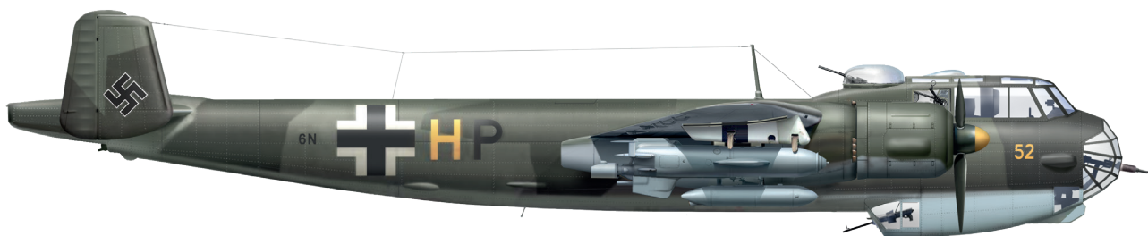
Do 217E-5 Wk-Nr 5552 6N-HP fitted with an Hs 293 remote-controlled glide-bomb and flown by Leutnant Horst Preißer of 6./KG 100 from Istres, France, in September 1943.
