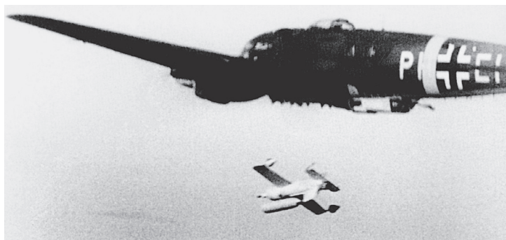
ABOVE An Hs 293 is launched over the Baltic during trials from He 111 carrier aircraft PH+EI attached to the E-Stelle Peenemünde's Test Section E4, which was responsible for the development and testing of remote-controlled guidance systems, radio communication and the use of television as a means of weapon control. PH+EI was fitted with extremely advanced equipment intended for television-guided launch trials with the Hs 293D. (EN Archive)
