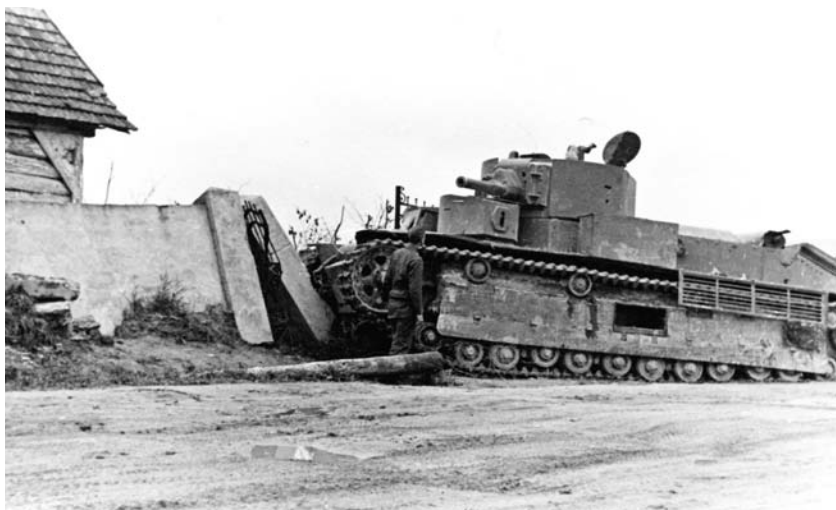
T-28 medium tank, a three-turreted machine designed for an infantry-support role. Its main turret mounted a 76.2mm cannon, while the two smaller ones each had one 7.62mm machine gun. It performed reasonably well during the Winter War with Finland in 1940. While outdated by 1941, it was the first vehicle of its class in the world to go into serial production in 1933.
