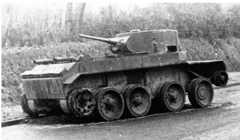
BT-7 light tank. The BT series of tanks, literally meaning “fast tank” (bystrokhodnyy tank), was developed to conduct break-through operations in depth. The basis for the BT series was the work of an American engineer, John Walter Christie. BT tanks operated in tracked and wheeled modes. This particular machine had its tracks removed to allow for faster movement on the road.
