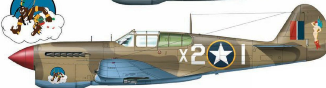
Curtiss P-40F, x2-1 , 86th Fighter Squadron, 79th Fighter Group, North Africa, 1943. Dupont 71-065 Dark Earth and 71-069 Middle Stone upper surfaces with 71-062 Azure Blue undersides; red spinner, white codes. Yellow outlined star on fuselage sides, above port and below starboard wings; unit badge on nose, 'angel' art on rudder. RAF style flash on fin
