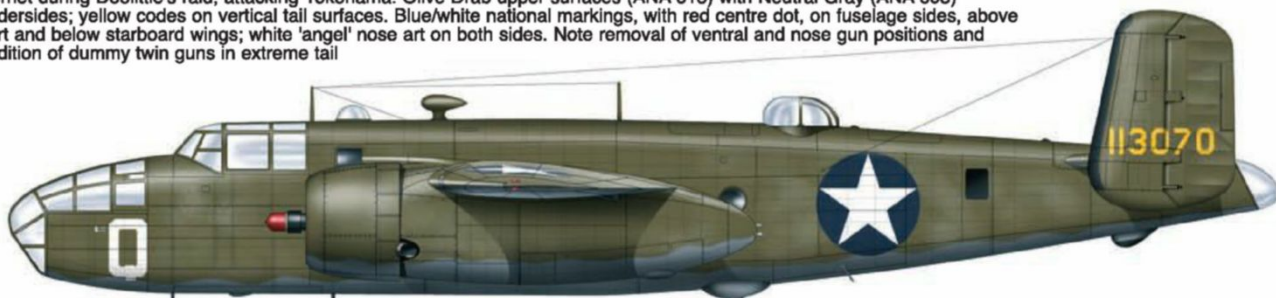
Above: North American B-25C-1 Mitchell, 41-13070/Q, 310th Bomber Group, Dodecanese. Very faded Olive Drab (ANA 613) upper surfaces with Neutral Gray (ANA 603) undersides. Blue/white star markings on both fuselage sides, above port wing and under starboard wing. White 'Q' on nose and yellow serial on fin
