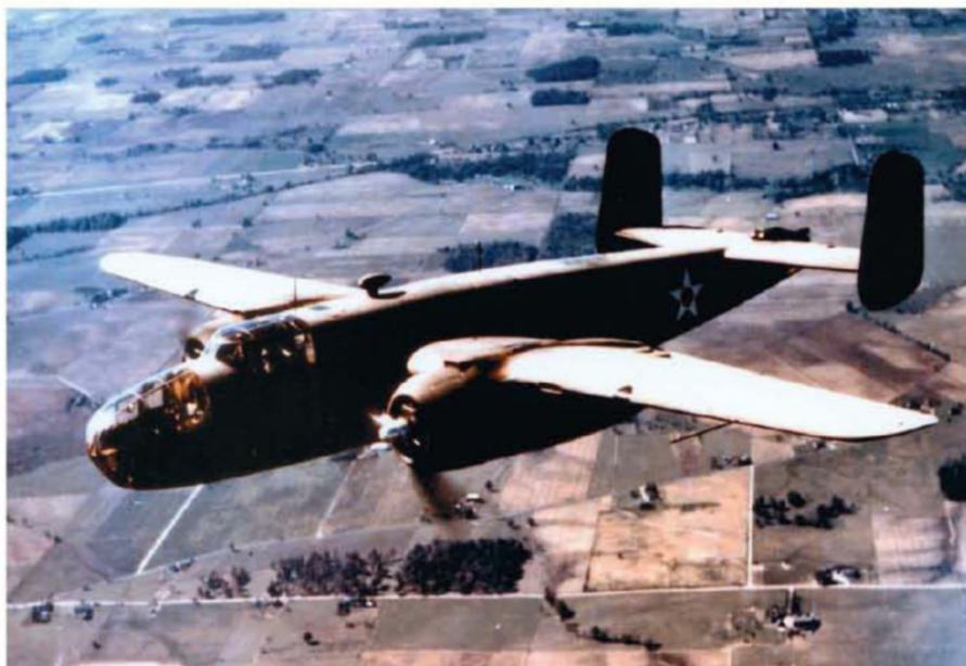
This rare photo of an early build B-25A shows the straight wing of these early machines plus the early USAAF 'meatball' national markings. USAAF/NARO
