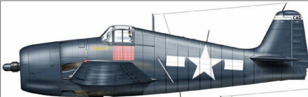
Grumman F6F-5 Hellcat, '7-F-1' of VF-7, USS Hancock (CV 19), 1944. Fuselage is in Non-Specular Intermediate Blue with Non-Specular Sea Blue top decking; top of wings and tailplane is Non-Specular Sea Blue. Undersides are in Non-Specular Insignia White; national markings on fuselage sides, above port and below starboard wings. Codes in white
