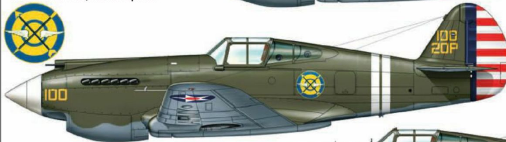
Curtiss P-40B , 17-35P, 33rd Pursuit Squadron, 35th Pursuit Group, USAAF, late 1941. ANA504 Olive Drab upper surfaces with ANA602 Neutral Gray undersides; red spinner, white nose section and two bands around rear fuselage. All lettering in black; US star markings on fuselage sides and above wings
