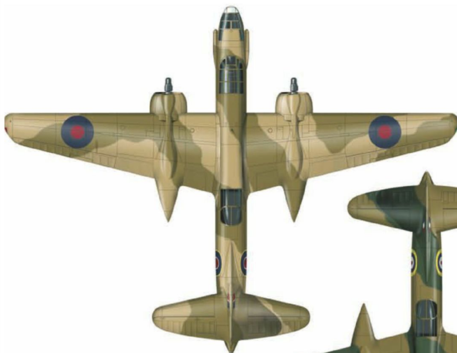
Right: Typical upper surfaces colour scheme for RAF and other Allied aircraft in Dark Earth and Dark Green. Standard 'B' style roundel is 45in diameter (1.14m)
