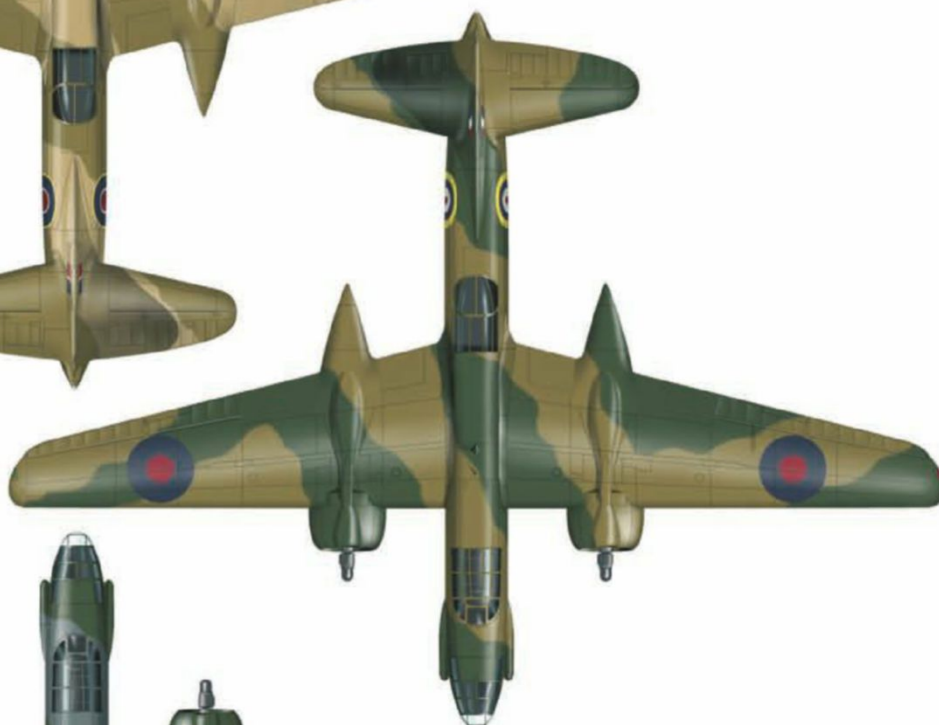
Left: Typical upper surfaces colour scheme for RAF and SAAF aircraft used in North Africa in Dark Earth and Mid-Stone. Standard 'B' style roundel is 45in diameter (1.14m)
