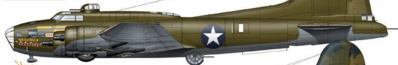
Boeing B-17F 41-24579/PU-F, 'Thumper', 360th BS, 303rd BG, 8th AF, USAAF, October 1942. Olive Drab with Medium Green dabbling on upper surface; Neutral Gray undersides. Fin lettering in yellow, codes in Neutral Gray
