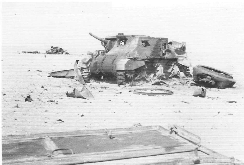
A 5th Tanks Grant destroyed during the Gazala battles, the blown-off turret and buckled hull plates bearing witness to the force of the internal explosions that destroyed it.
