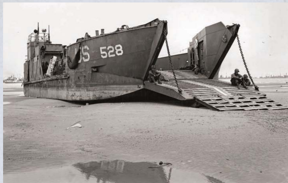
Weighing in at just over three hundred thousand pounds, LCT-528 sits high and dry on Utah Beach while crewmen relax on her bow ramp waiting for the high tide to return. This landing craft was built by Bison Shipbuilding Corporation of North Tonawanda, New York, in 1943. U.S. Navy photograph, now in the collections of the US National Archives 80-G-253009
