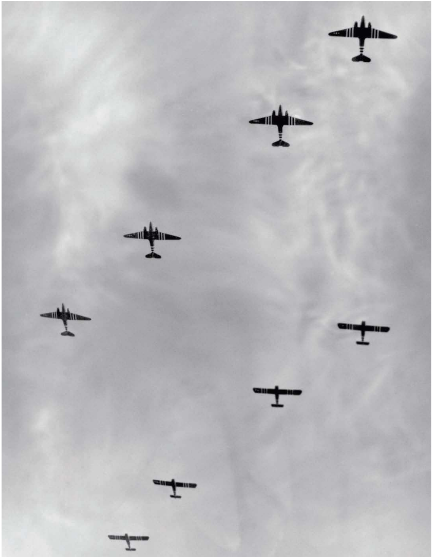
C-47 Skytrain transport aircraft tow Waco CG-4A gliders to Normandy on June 7, 1944. Although the larger British Horsa glider offered greater carrying capacity, the CG-4A was nevertheless capable of hauling a 57mm antitank gun, a 75mm PAK Howitzer, a Jeep, or thirteen fully armed troops.
