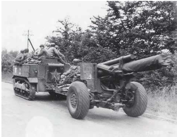
LEFT: An M1 155mm howitzer from the 34th Field Artillery Battalion, 9th Infantry Division is towed on the N-13 by an International Harvester M5 (13t) High-Speed Tractor. The M5 was standardized in October 1942 from the T21, a vehicle based on the tracks and suspension of the Stuart light tank. International Harvester started production of the vehicle in 1942. National Archives and Records Administration/U.S. Army Signal Corps 111-SC-190385
