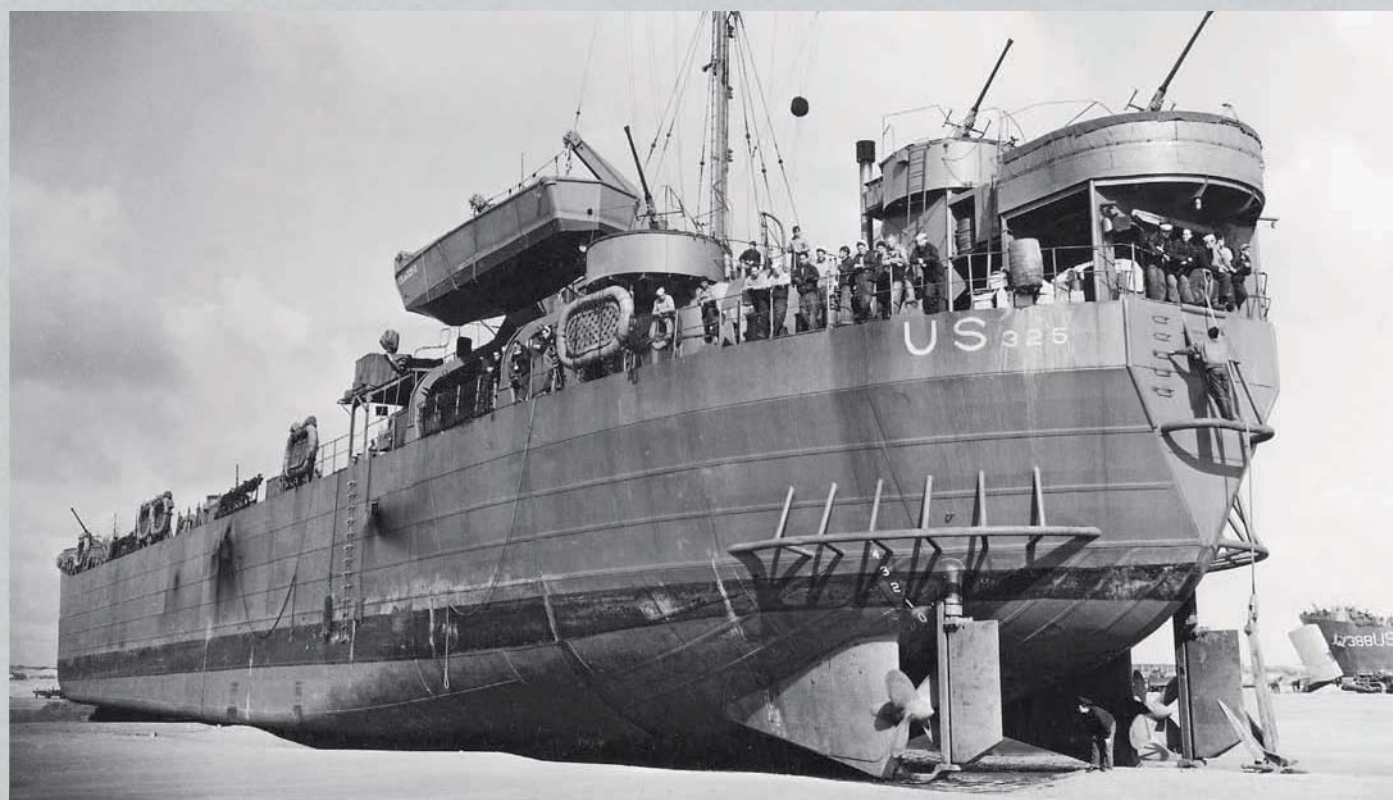
ABOVE: LST-325 sits high and dry on Utah Beach on Monday, June 12, 1944. In this photo, it is easy to see the roll-on/roll-off capability that made the LST such a versatile and effective weapon. LST-325 survived the war and was ultimately given to the Hellenic Navy in 1964. In early 2001, the ship returned to the United States and is now the USS LST Ship Memorial Museum in Evansville, Indiana. Official U.S. Navy photograph, now in the collections of the National Archives 80-G-252795 BELOW: LST-325 (left) and LST-388 (right) are beached at low tide during resupply operations on Utah Beach on June 12, 1944. Visible here are four of the ship's 40mm anti-aircraft guns and one of her LCVs suspended from its lifting davits. Official U.S. Navy photograph, now in the collections of the National Archives 80-G-252799
