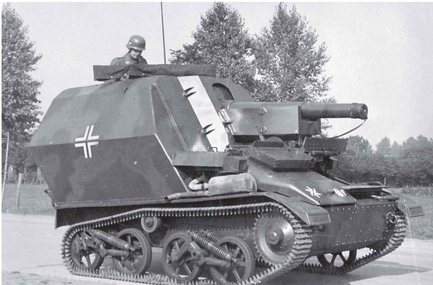
A most improbable marriage was this mounting of a le FH16 105mm howitzer on the chassis of a British Mk VI light tank captured in 1940.
