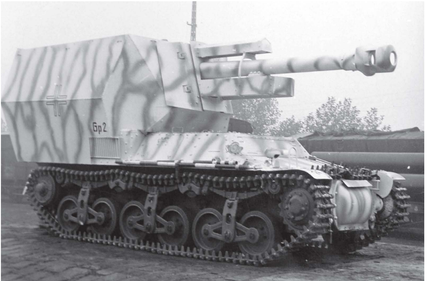
German ingenuity led to the creation of hybrid vehicles with German weapons mounted on the chassis of captured Allied vehicles. This example is a leFH18 105mm howitzer mated with a French Lorraine fully-tracked armoured ammunition vehicle.
