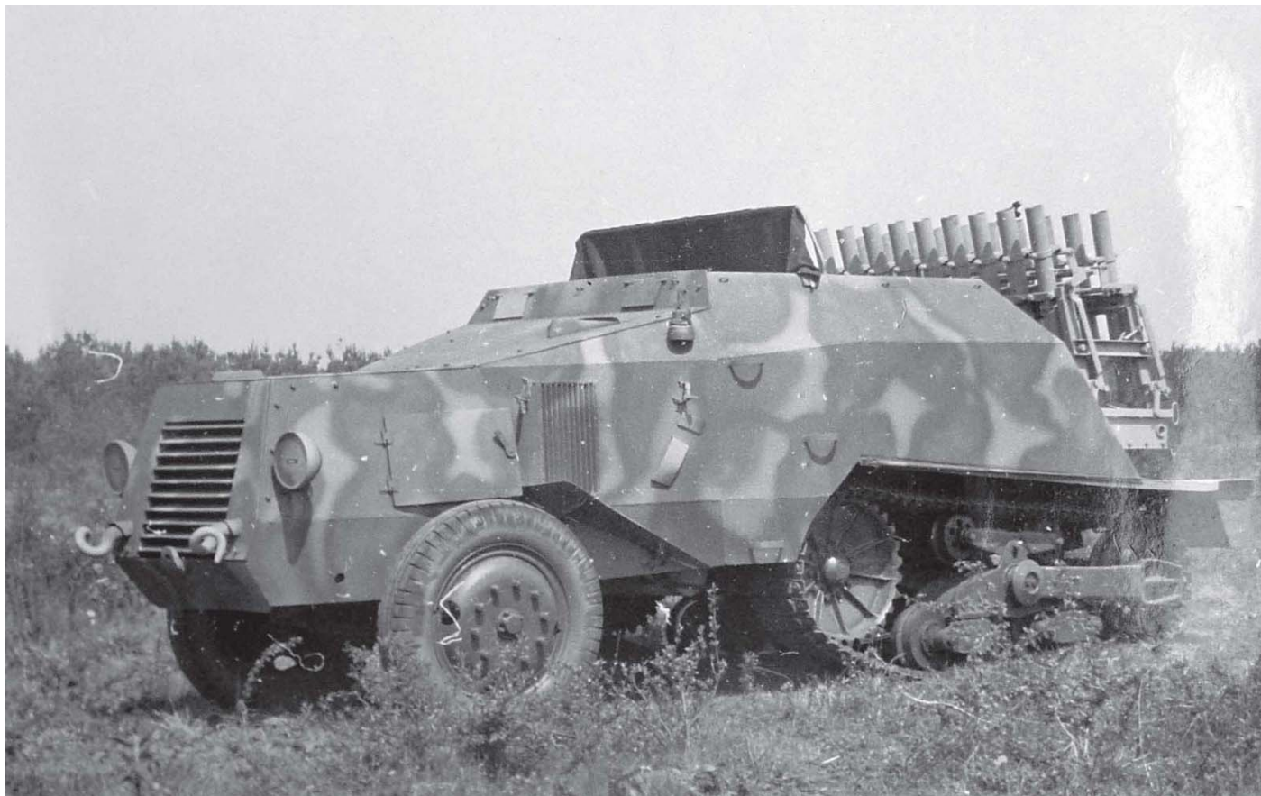
Another hybrid was this French Somua half-track armed with multiple 80mm mortars.
