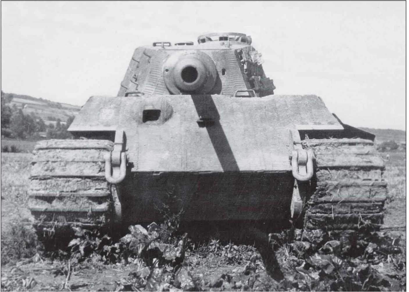
The Tiger II was an improved model with thicker armour that was sloped to provide additional protection. Only twenty-five of these vehicles served in Normandy.
